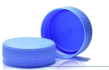
During the recycling process, plastic closures are shredded together with PET bottles. Since polyolefins are less dense (density=0.90 g/cm<sup>3</sup> to 0.96 g/cm<sup>3</sup>) than water (1 g/cm<sup>3</sup>), shredded closures float on the surface and are separated from the more dense PET flakes (1.35 g/cm<sup>3</sup>), which settle at the bottom of the sink-float tank.
