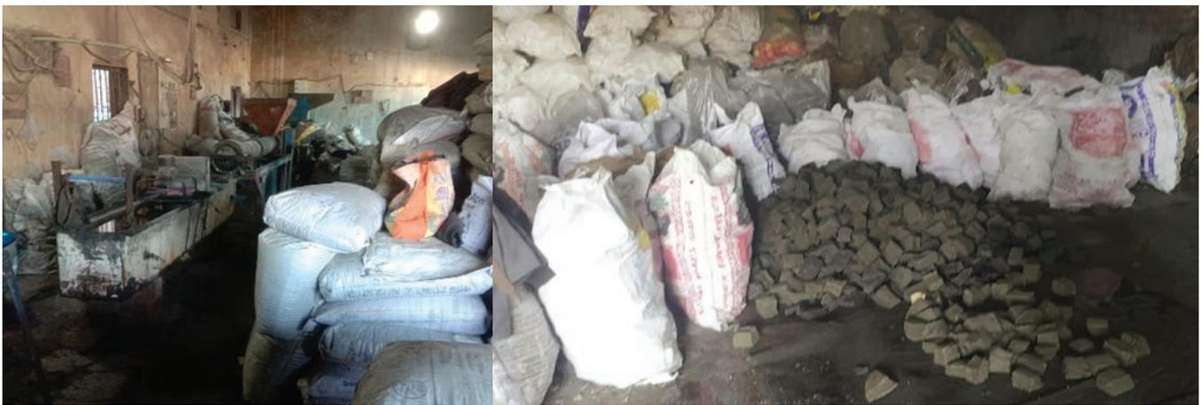
Figure 5: A Type 2 recycling unit manufacturing recycled blocks from mixed plastics
